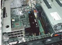
After removing one of the original processors (for details, refer to your motherboard manual).
